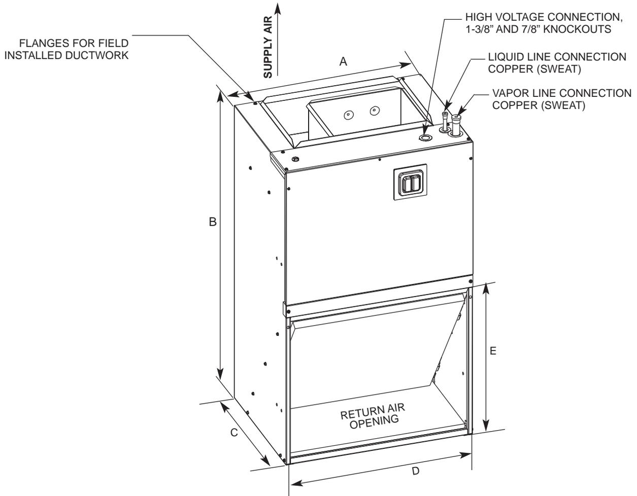
ALL UNITS ARE CONFIGURED FOR VERTICAL UPFLOW. UNITS CANNOT BE INSTALLED IN ANY OTHER CONFIGURATION.
