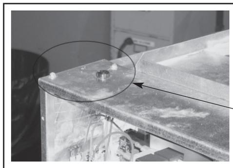
Remove 6 Sheet Metal Screws From Top Plate
